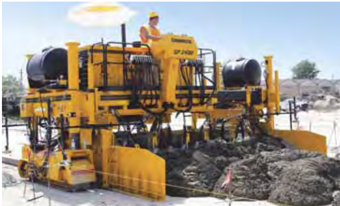
The GP-2400's pedestal console shifts out for paving and retracts back in for minimum shipping requirements.
